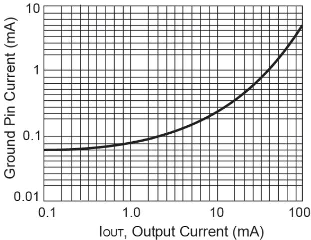
**Figure 3. Ground Pin Current vs. Output Current**
