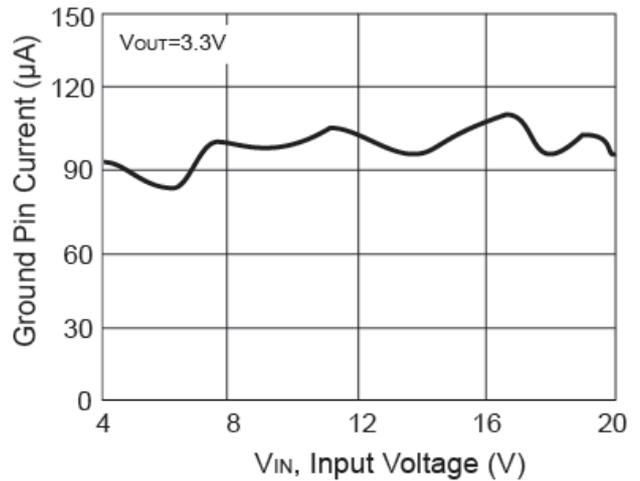
**Figure 4. Ground Pin Current vs. Input Voltage**
