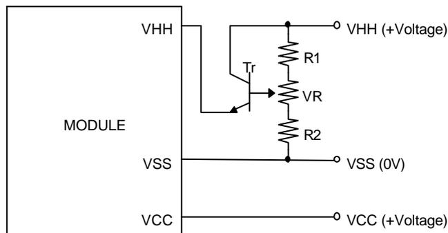
$$R_1 + R_2 + VR = 10 \sim 20K\Omega$$
