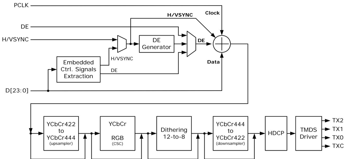
**Figure 3. Video data processing flow of CAT6612**
