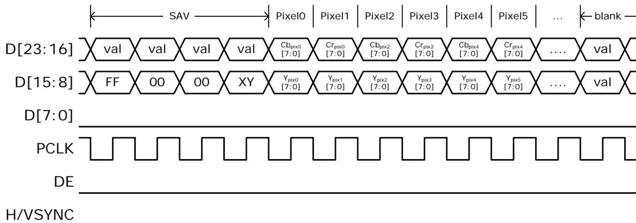
**Figure 7. 16-bit YCbCr 4:2:2 with embedded syncs**
