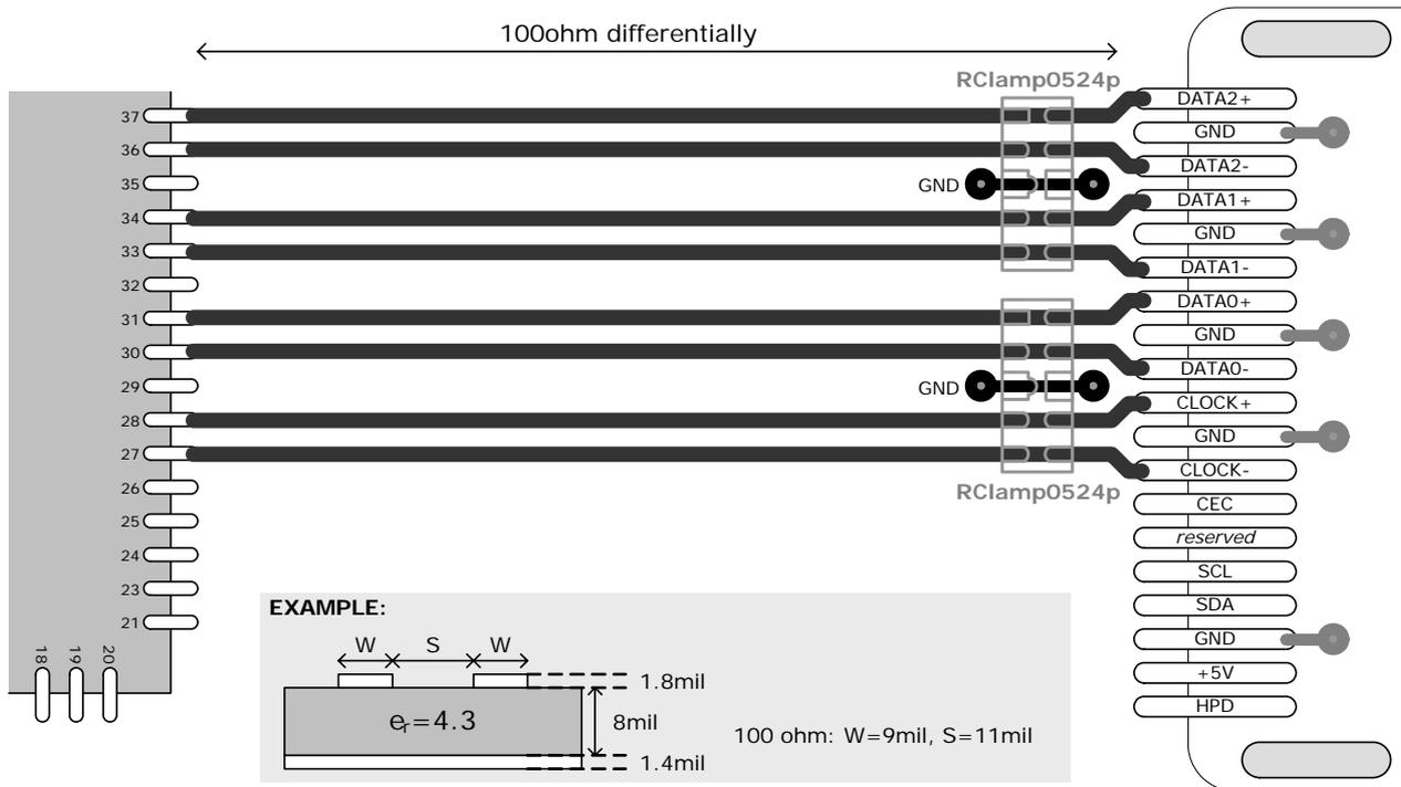
**Figure 11. PCB layout example for high-speed transmission lines with RClamp0524p**
