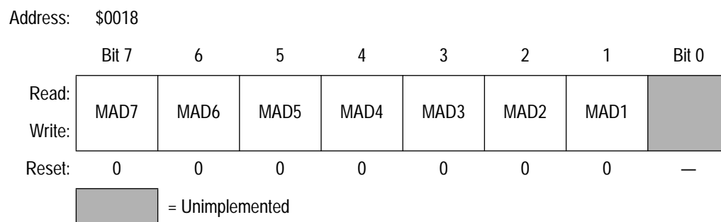
Figure 11-3. M-Bus Address Register (MADR)
