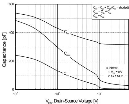
**Figure 5. Capacitance Characteristics**
