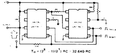
Figure 13. Cascaded Operation of Two XR-2242 Timer Circuits
