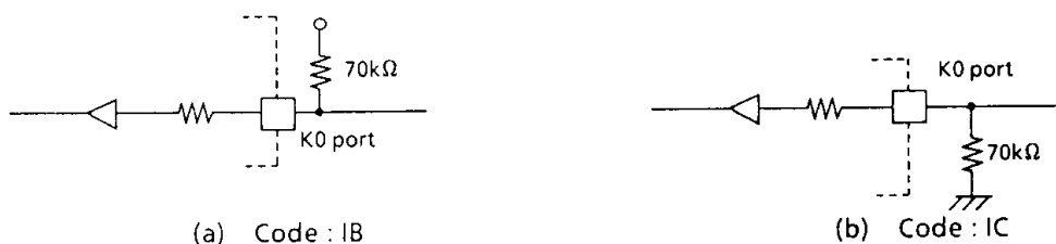
Figure 2. I/O code and external circuitry
