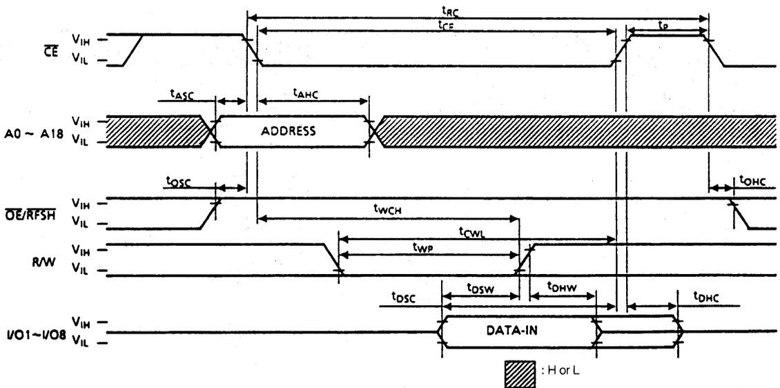
Write Cycle 2 ( $\overline{OE}$  Clocked or Fixed Low)
