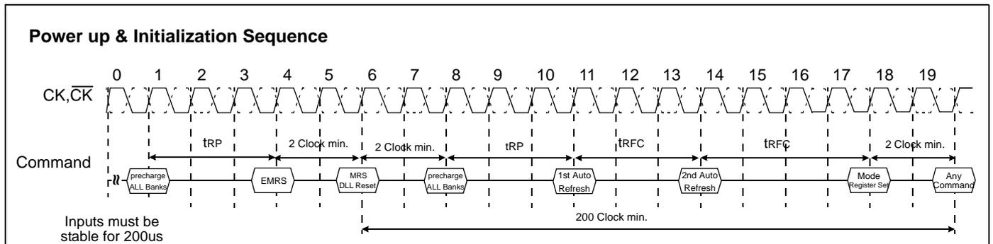
\* When the operating frequency is changed, DLL reset should be required again.
