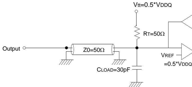
(Fig. 1) Output Load Circuit
